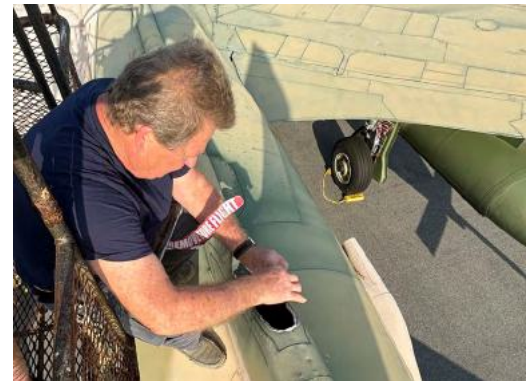
Charlie Hammer applies adhesive to spine of F-105 for replacing missing cover.
