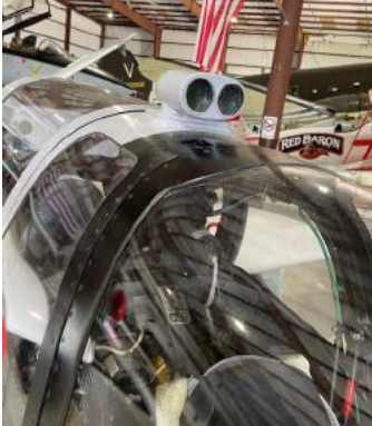
Binocular periscope on the Fouga Magister
