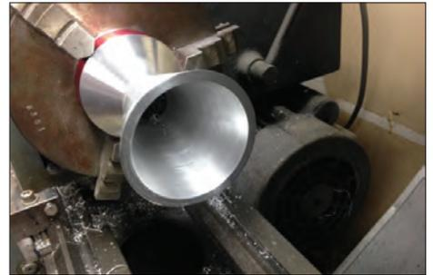
*The lathe compound slide is set over to 17 degrees and the boring bar is advanced at that angle to cut the inside taper.*
