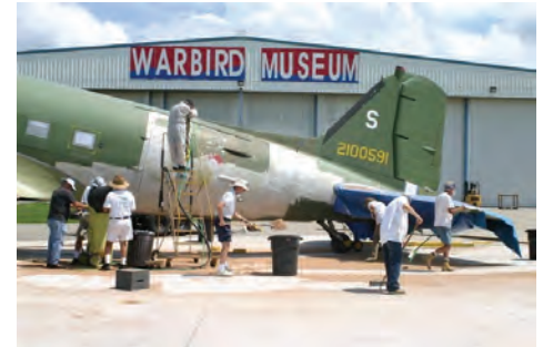
Tico Belle being stripped with crushed walnut shells..
