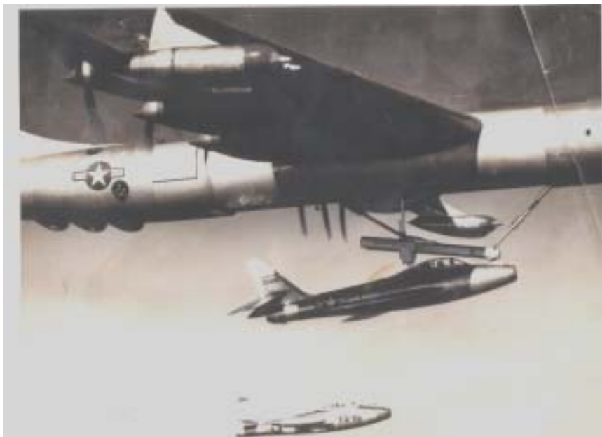
F-84G hooking up to the mother-ship B-36 during early FICON tests
