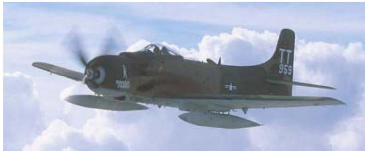
(Left) The Douglas A1-D Skyraider, flown by Mike Schloss, has a prop 13.5 feet in diameter. It was designed to replace the Dauntless Dive Bomber and
