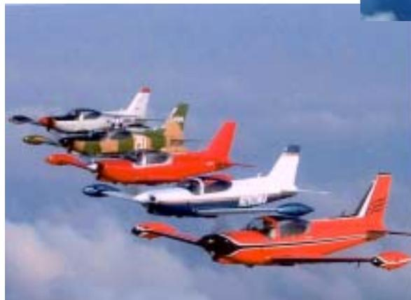
The Siai-Marchetti SF.260 (left) flown by the Marchetti Maverick team has a 260 HP Lycoming engine and a top speed of 250 mph. It is fully aerobatic and can be configured with external racks for bombs, rockets, or a machine gun.
