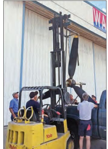
5-29-14 Loading the TBM propeller onto Tom Reilly's truck. The prop will be tested, magna-fluxed, balanced and certified for flight
