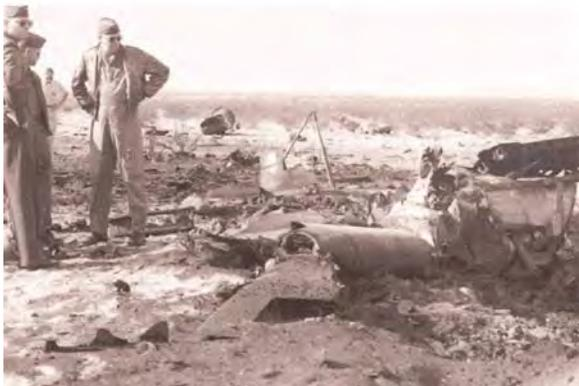
Looking at this wreckage created a warning to me as I was going to be assigned the task of identifying the flight regime where the aircraft approached the point where the “pitch-up” occurs and from where no recovery is possible. The U.S.A.F. had bought the F-101B and the company had designed a very conservative stall avoidance system which compromised the full maneuvering capabilities of the aircraft.
